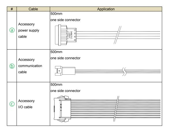
Wire Specification Power supply cable : AWG18 UL1015 (105°C / 600V)
