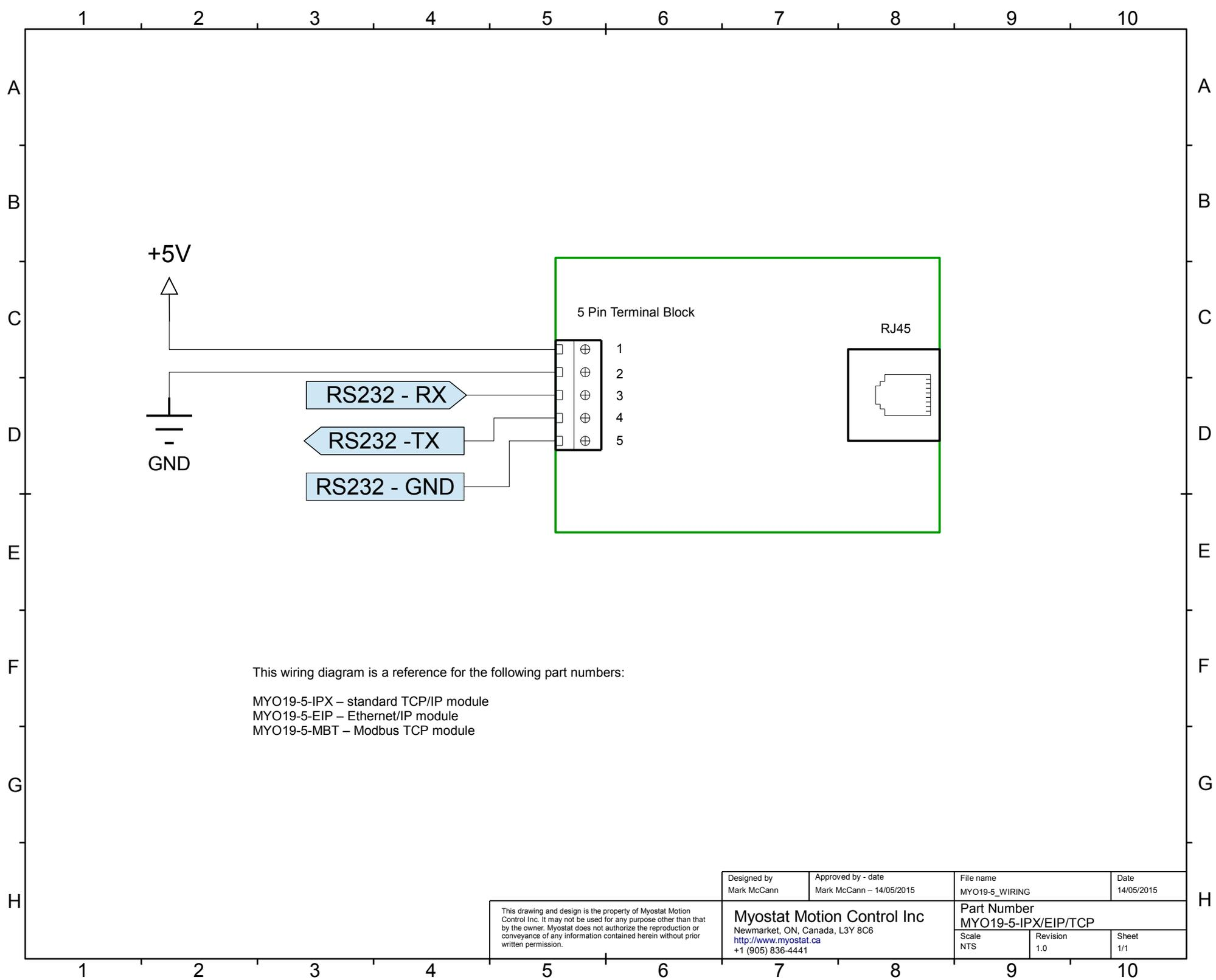
This wiring diagram is a reference for the following part numbers:
