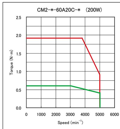
\* Input Voltage is AC200-240V
