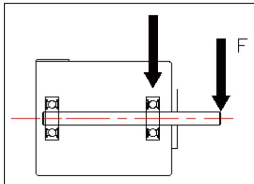
Moment load is applied ( see the illustration in the right) to the motor shaft that is overhung. A tension force is applied to the top half of the shaft and compression forced is applied to the bottom half of the shaft. During the shaft rotation, these opposite forces alternate and stress the shaft, and continued rotation over the long term could result in break.
