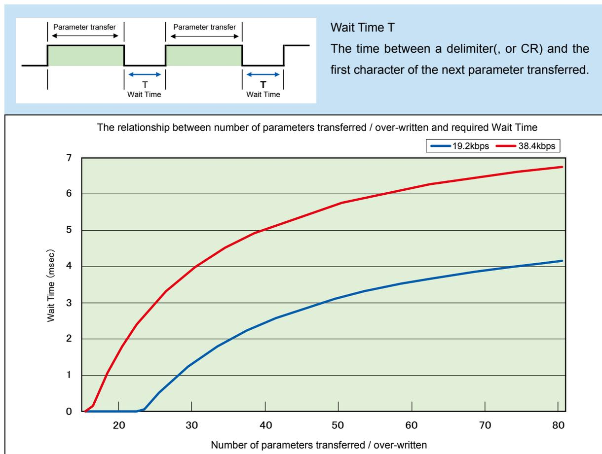
\* Wait Time will not be required in 9600 bps. But the communication will be more stable if 1msec time interval is set between each transferred parameter.
