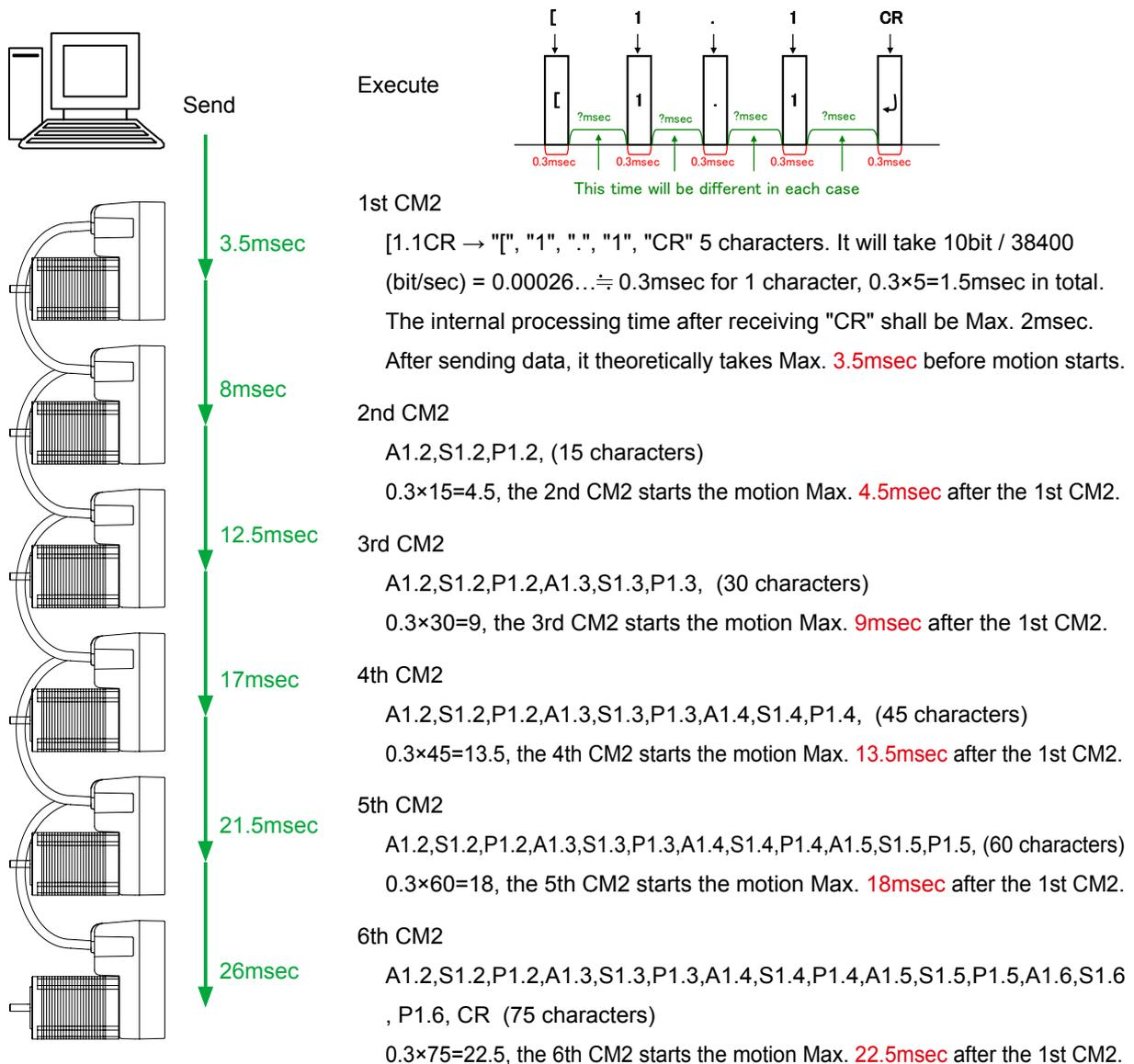
\* By defining only the "A" and "S" data for ID1 ~ 6 in the first line and "P" data for ID1 ~ 6 in the second line, the time delay between each motor shall be shorten to approximately **1.5msec**.
