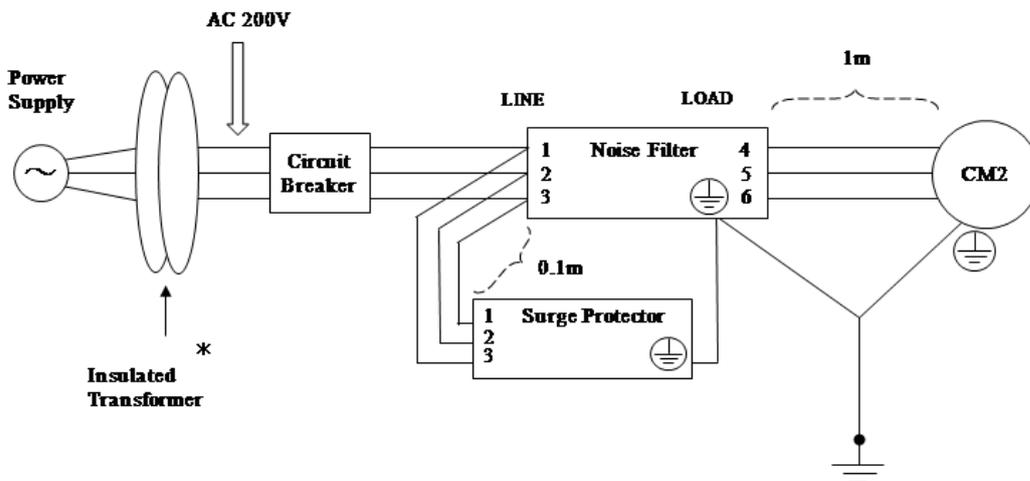
\* Use an isolating transformer when necessary
